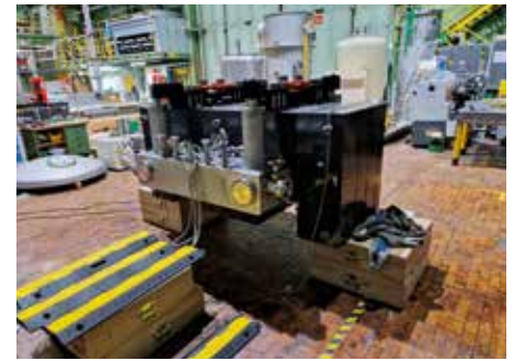
Fig. 7: Superconducting magnet of the magnetic heater in current test at KIT with iron yoke
