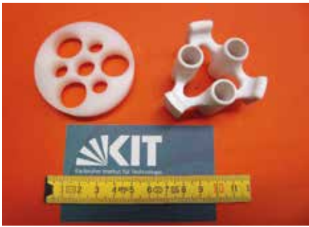
Fig. 4: PE disk insulator (left) and printed PLA support insulator (right)
