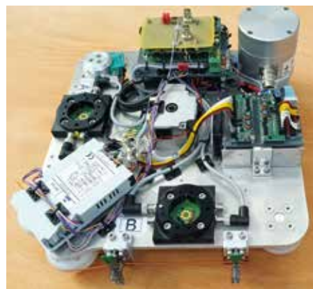
Fig. 1: Electronics side of the winding hand. Bottom left: PID tension controller. Further clockwise: Docking flange for robot, rotary encoder for length measurement, electronics for S7 connection, tensile force sensor, motor control. In the centre: servo motor.
